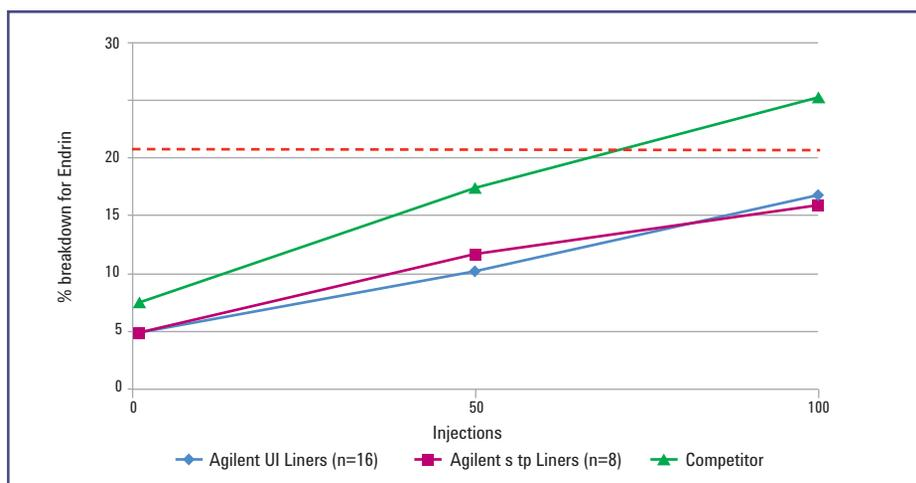
Agilent Ultra Inert Liners with wool are superior vs. the competition as shown in this endrin breakdown comparison.
