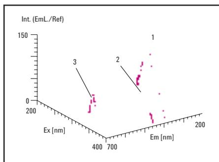
The total fluorimetry spectrum of the 50 mM borate buffer pH 9.2 verifies that the solution is free of fluorescence-active impurities (1 and 2 = Rayleigh stray light of zero and first order, 3 = Raman stray light).
