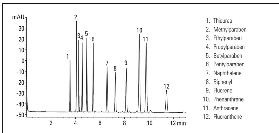
Capillary Electrochromatography of parabens and aromatics
