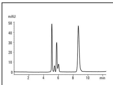
CZE analysis of a peptide mixture using pre-made 50 mM sodium phosphate buffer, pH 2.5
