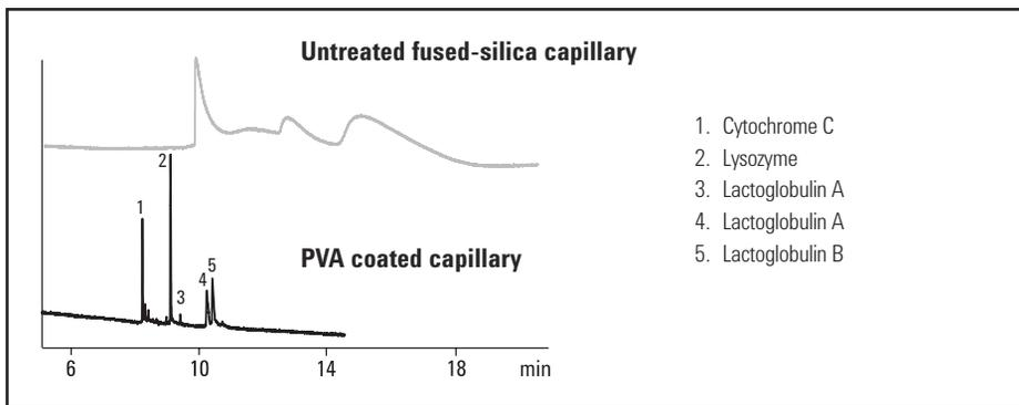
Use of PVA coated capillaries to reduce protein adsorption
