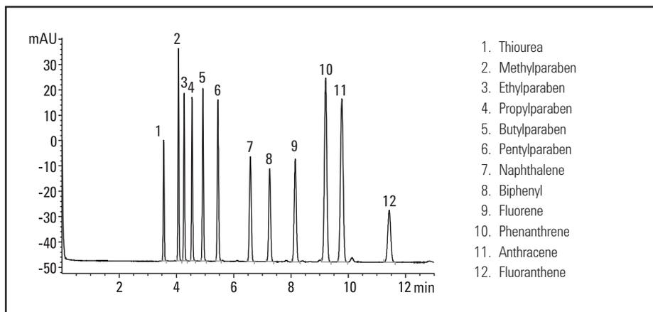
Capillary Electrochromatography of parabens and aromatics
