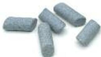
Ceramic homogenizer for 50 mL tubes, 5982-9313
