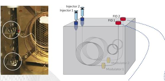
Use of two INSIGHT modulators in a dual-channel configuration immediately doubles productivity, resulting in a swift return on investment. This is illustrated for environmental monitoring of total petroleum hydrocarbons (TPH) using the 'stencil' feature in SepSolve's ChromSpace software.
