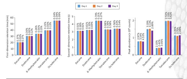
Excellent repeatability of retention times is aided by the use of a dedicated EPC for each column. The charts show <1% RSDs for first-dimension and second-dimension retention times, and <5% RSDs for peak abundance, for 24 injections of diesel over 3 days (n = 8 injections/day).
