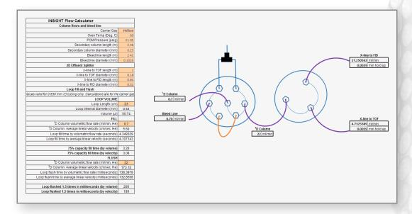
Simplify your GC×GC method development by using the flow calculator that comes as part of the INSIGHT software package.
