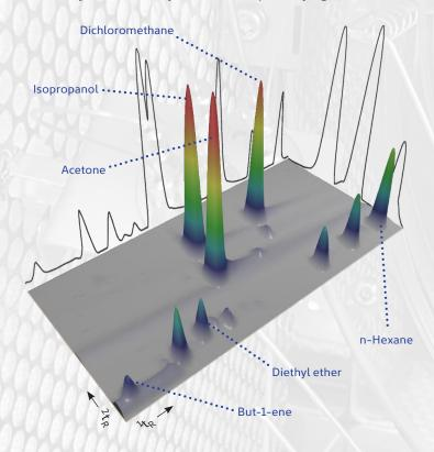
Efficient modulation of compounds <C<sub>6</sub> using INSIGHT provides sharp and symmetrical peaks for volatiles in blood.
