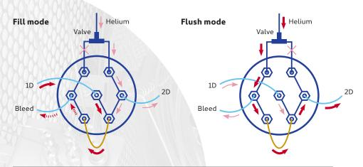
INSIGHT uses a two-stage process involving the sample loop (orange) to achieve effective modulation. In fill mode, the primary column eluate enters the sample loop (with any overfill directed to a bleed line), while the modulation valve directs auxiliary carrier gas to the secondary column. The valve then switches, and the contents of the sample loop are flushed rapidly on to the secondary column as a narrow chromatographic band.
