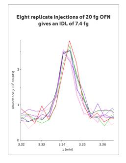
Improved detection limits (<20 fg OFN) with full spectral information means a wide range of trace-level species can be detected in a single analysis. BenchTOF2 also allows retrospective searching for new compounds of interest.
