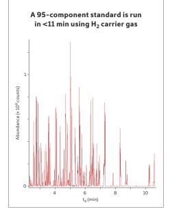
BenchTOF2 is fully certified for use with hydrogen carrier gas. The result is faster chromatographic separations, reduced running costs, faster return on investment, and mitigation of gas supply issues.
