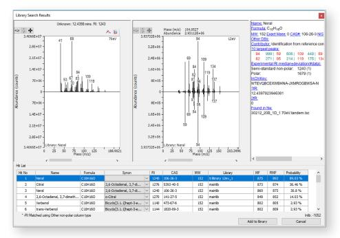
Dual library searching adds confidence to identification, by using both 70 eV and soft EI spectra to find the top library match across both data blocks in a single workflow. In this case, the 12 eV data confirms the isomer as neral. ChromSpace<sup>®</sup> software offers easy batch addition to spectral libraries, simplifying the creation of soft EI libraries.
