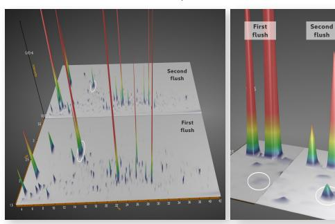
The comprehensive analytical resolution of GC×GC combined with BenchTOF2 and Tandem Ionisation easily uncovers key differences in the aroma profiles of two tea samples, revealing *trans*-2-hexenal (with a strong 'green' aroma) in the lower-quality 'second flush' teas.
