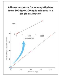
Extended dynamic range across five orders of magnitude allows accurate quantitation of high-concentration compounds, while maintaining low detection limits. This removes the need for dilutions or repeat analyses.
