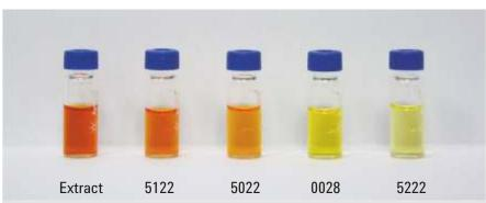
Extract and four different dispersive clean up; 5222 kits removing more pigments and consequently enhance column, liner life & source cleaning. The recovery for the majority of the compounds is between 70-120%
