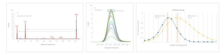
Once you have chosen the unique MRM transitions, collision energies (CE) should be ramped systematically to determine the maximum signal produced with good peak shape. Similarly, by plotting abundance versus collision cell voltage, a clearer picture of the effects of MRM collision energy emerges. In this example, the ideal CE values are 16 and 32 V.
