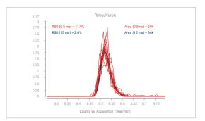
At lower instrument dwell times (typically <5 ms), ion beam sampling becomes less precise due to the insufficient number of ions involved in the measurement. In the context of chromatographic peak area, lower dwell times can increase the uncertainty (% RSD) of measurements within a set of replicates. The figure compares the results for the same analyte at the same concentration, but with different dwell times—emphasizing its effect on % RSD.
