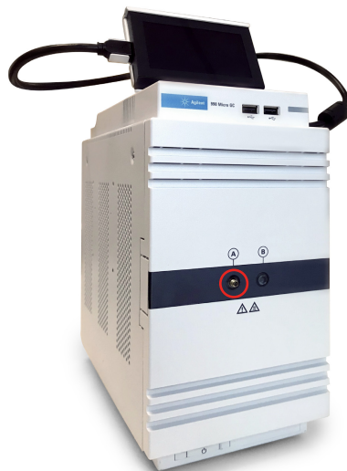
Figure 1A. Two-channel NGA analyzer. The red circle indicates the sample inlet.
