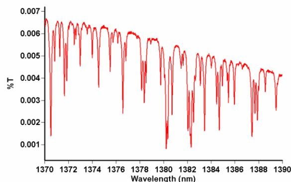
Figure 2: Water vapor transmission spectrum collected on a Cary 6000i spectrophotometer
