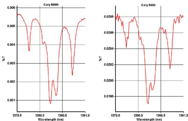
**Figure 3:** Resolution of the 1380 nm water vapor peak collected on a Cary 6000i and a Cary 5000 spectrophotometer
