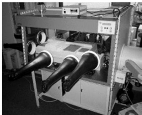
**Figure 1.** The Cary Deep UV and nitrogen-purged glovebox
