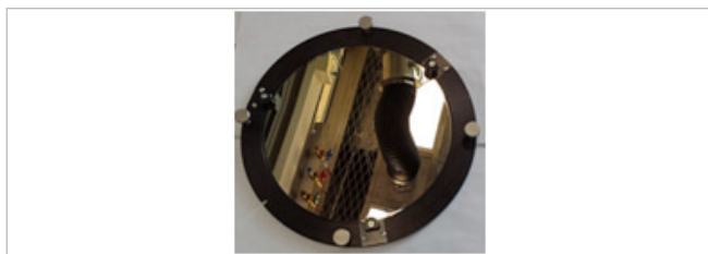
Figure 3. A 200 mm diameter precut wafer mounted in the 8" sample holder that attaches into the Solids Autosampler.
