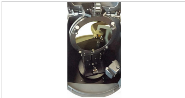
Figure 4. Front view of the Cary 7000 UMA sample compartment with the Agilent Solids Autosampler installed and the 200 mm diameter coated wafer mounted into the autosampler.
