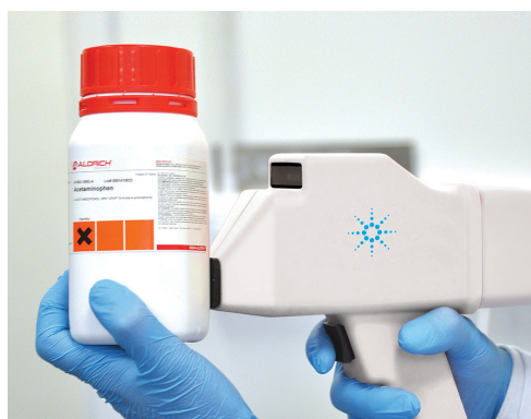
Figure 1. RapID verification system identifying a material through a plastic container.
