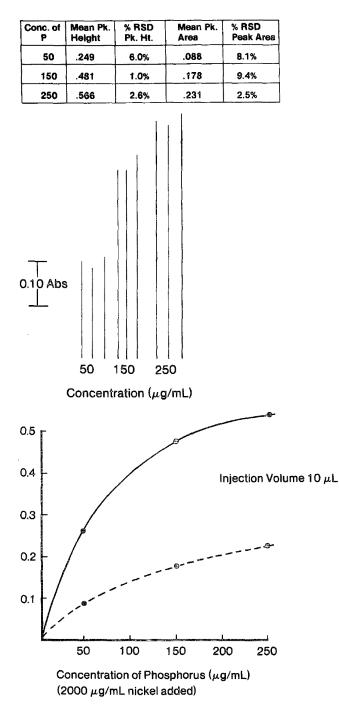
Figure 3. CRA-90 Determination of phosphorus in oil.
