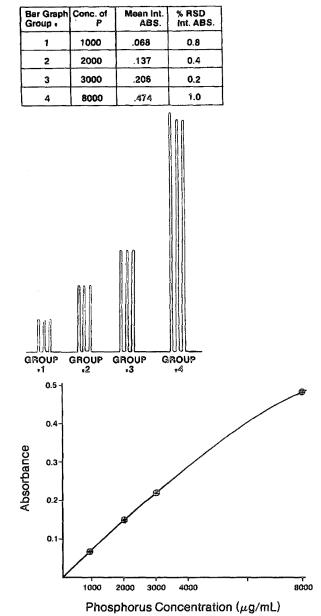
Figure 1. Flame determination of phosphorus in organic matrices.
