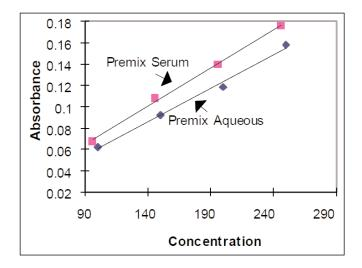
Figure 2. Serum standard addition calibrations.
