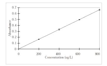
Figure 1. Selenium calibration graph.
