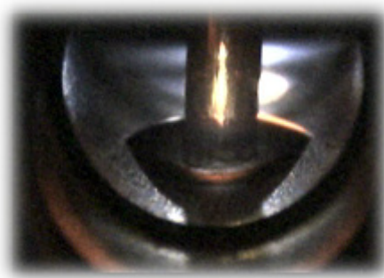
Figure 1. The view inside the tube, using the integrated camera. This shows the probe dispensing the sample into the tube.
