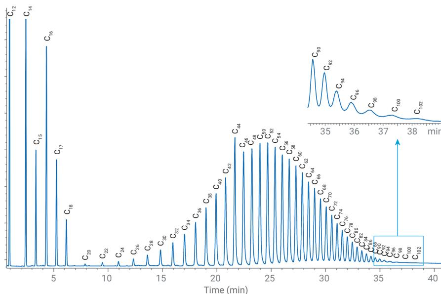
**Figure 1.** D6352 calibration showing elution of  $n$ -C<sub>12</sub> to  $n$ -C<sub>102</sub> paraffins. The inset shows details of paraffin detection greater than  $n$ -C<sub>90</sub>.
