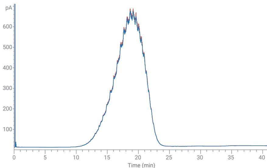
**Figure 4.** Overlay of duplicate analyses of a vacuum gas oil samples. Table 4 shows the results from the Agilent SimDis software engineering report along with the repeatability (r) performance compared to the ASTM D6523 repeatability limits.
