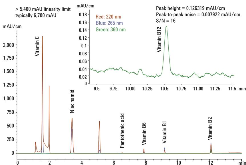
Figure 6. Analysis of vitamins with an Agilent 1260 Infinity HDR DAD.
