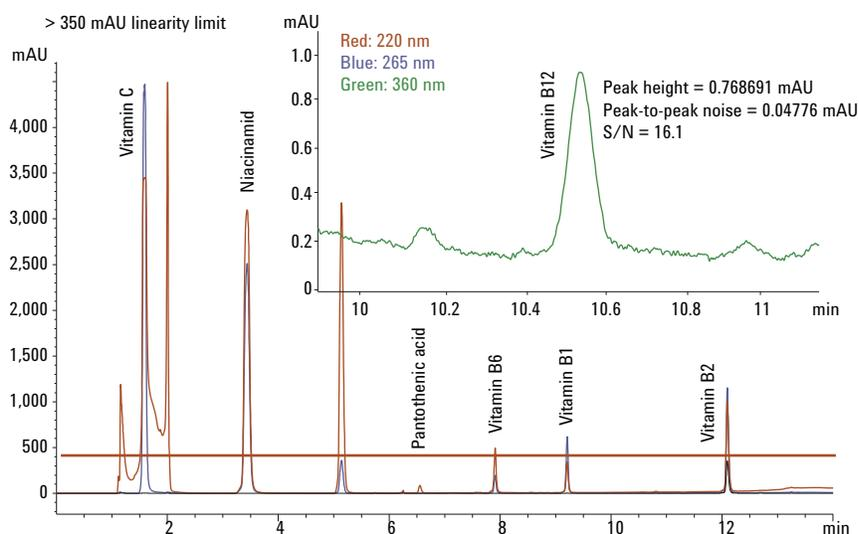
Figure 5. Analysis of vitamins with an Agilent 1260 Infinity DAD with a 60-mm path length cell.
