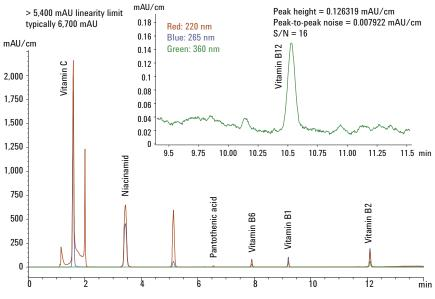
Figure 6. Analysis of vitamins with an Agilent 1260 Infinity HDR DAD.
