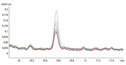
Figure 7. Decomposition of vitamin B12 over time.
