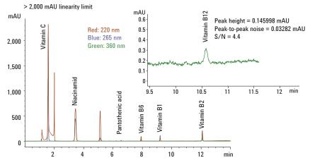
Figure 4. Analysis of water soluble vitamins with an Agilent 1260 Infinity DAD with a 10-mm path length cell.
