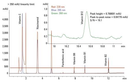
Figure 5. Analysis of vitamins with an Agilent 1260 Infinity DAD with a 60-mm path length cell.
