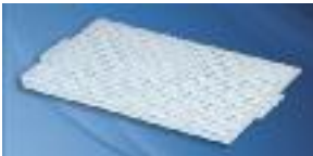
384-well plates and mats Notches on A24 and P24 side
