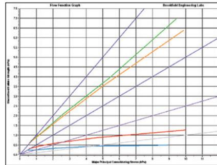
Flow Function test produces graphs of powder flow behavior which show:
