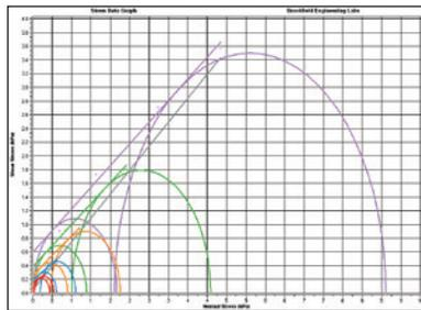
Stress data output screen captures "normal stress" and "shear stress" values and plots data in graphical format (calculates Mohr Circle Failure Loci).
