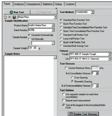
Main screen provides choice of basic tests:
