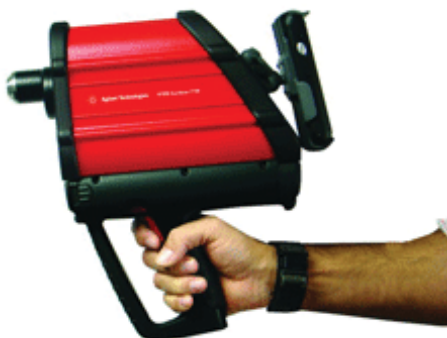
Figure 1a. Agilent 4100 ExoScan FTIR system in hand-help operation for at-site use. When used for at-site analysis of coal, all instrument functions are executed using the attached PDA. An automated, on-board method for the verification of coal quality is initiated by simple touch screen commands and results are clearly displayed on the PDA.
