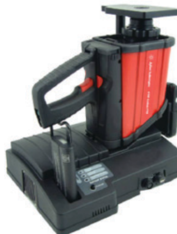
Figure 1b. Agilent 4100 ExoScan FTIR system mounted in a docking station for fixed use.
